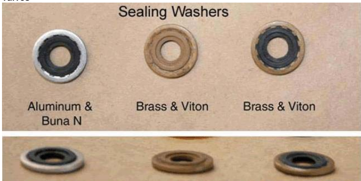
Figure 2: Examples of some sealing washers available for CGA 870 Style medical post valves.
