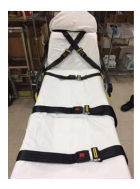
The mattress on the stretcher comes in two pieces to accommodate the shoulder straps. While this may make it slightly more inconvenient to put a sheet on the entire mattress, the design and location of the shoulder straps affords the maximum crash safety for the patient. A sheet can be placed on the main part of the mattress, and a towel can go on the head-rest / pillow portion.
