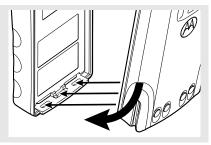
2 Press the top of the battery against the radio until both latches click into place.
